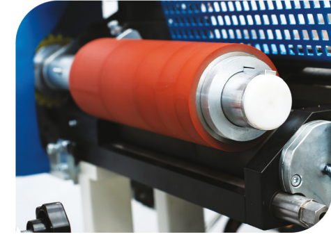
Özel Olarak Tasarlanmış PP, Finish Folyo, Doğal Kaplama ve Laminat Malzemelerine Tutkal Uygulayan Merdane Glue Application Roller is Designed for special production of PP, Finish Folio, Natural Coating and Lamination
